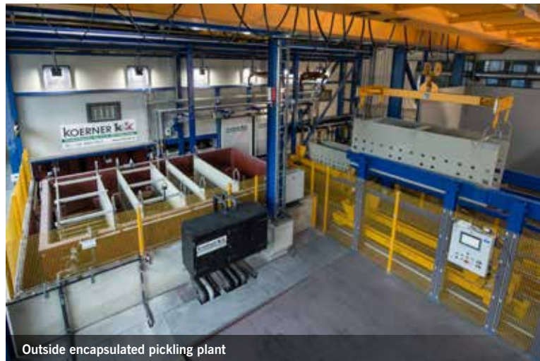
Pickling tank for HF + HNO 3 Tank dimensions: 13.9 x 1.5 x 3.3 m
