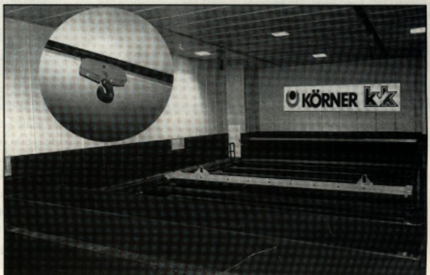
Figure 1. Transport units are not exposed to fumes; only hooks are inside the enclosure
